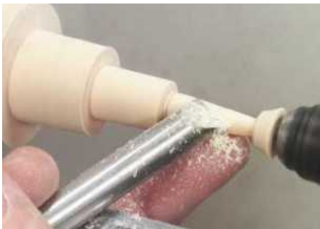
▲ Pic.4 It's that time again to support it with your finger. My left finger is underneath the toolrest and just touching the wood; this will help you to turn very thin and is safe as long as your digits are behind the wood
